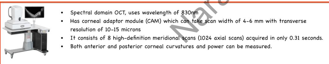
**Figure 18:** Optovue RVue spectral domain OCTs
